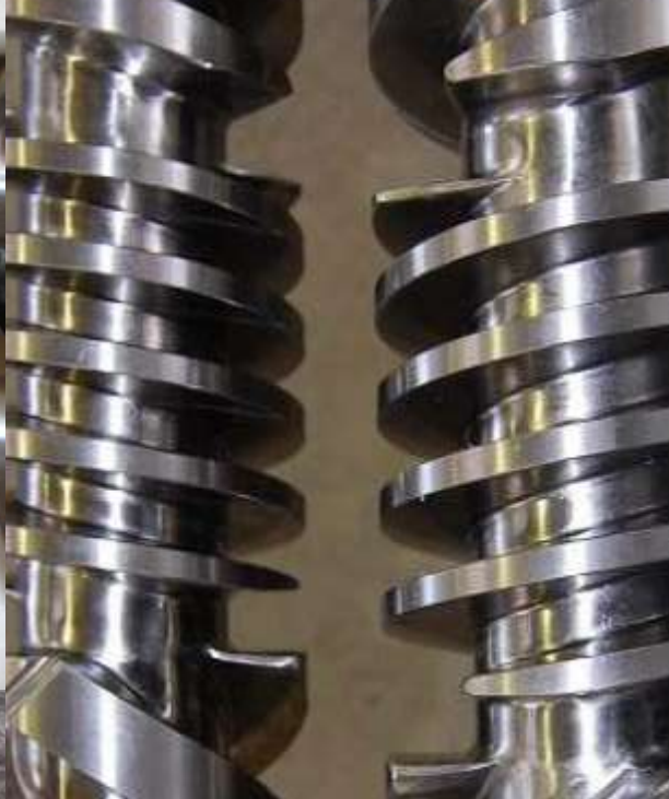
Tungsten Carbide (WC) Coated twin screw at Raj Engineering Works
